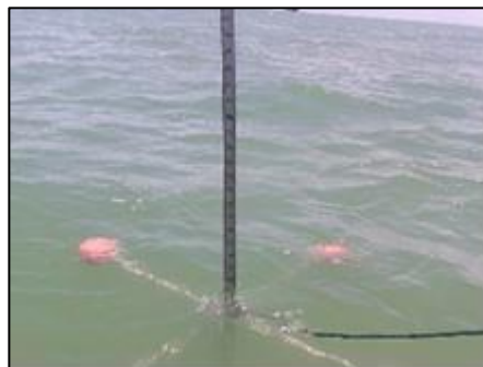
Figure 3. The Pole Measuring Wave Height
